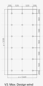
V3. Max. Design wind load: 3.5 kN/m²
