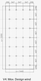
V4. Max. Design wind load: 5.5 kN/m<sup>2</sup>
