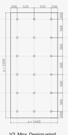
V3. Max. Design wind load: 1 kN/m²
