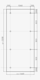
V1. Max. Design wind load: 1.5 kN/m²
