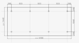
H1. Max. Design wind load: 0.5 kN/m<sup>2</sup>
