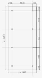
V1. Max. Design wind load: 0.5 kN/m²
