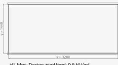
H1. Max. Design wind load:  $0.5\,kN/m^2$
