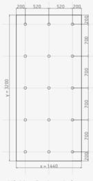
V2. Max. Design wind load: 3.0 kN/m²
