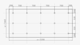
H2. Max. Design wind load: 3.0 kN/m²
