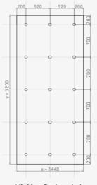
V2. Max. Design wind load: 1 kN/m²
