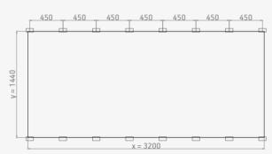
H1. Max. Design wind load: 2.8 kN/m<sup>2</sup>
